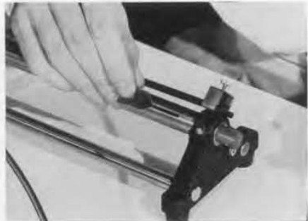
Figure 12. Tool for removing sample is also furnished.
